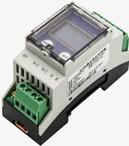
The LoRa Serial Converter CC32LR is an RS-485 device that uses an enhanced LoRa module, works in the data transmission mode, supports various protocols, and can realise long-distance wireless network communication by joining the LoRa network.
