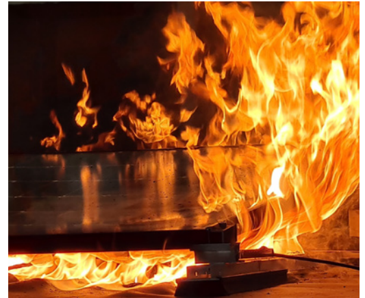
Arc-induced fire under flat roof mounted solar at ZAG fire testing laboratory
